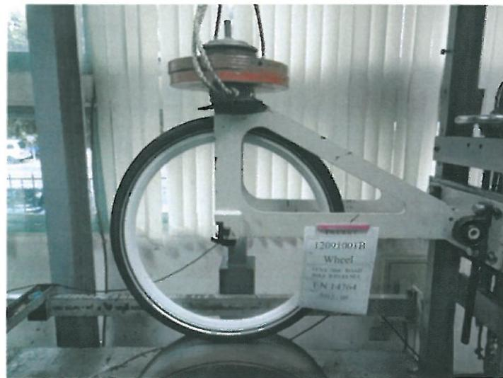
Fig. 2 Wheel dynamic test .
